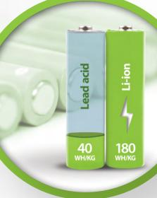
Lithium-ion vs Lead Acid
